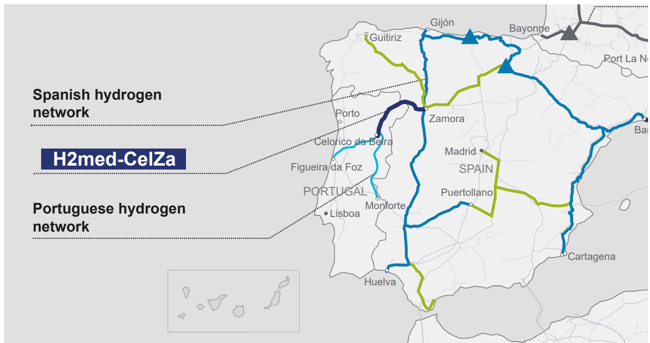
The Spanish hydrogen transmission network is structured around two main corridors. The first includes the Cantabrian coast corridor, the Ebro Valley corridor and the Levante corridor. The second includes the Via de la Plata corridor, connected to the Puertollano hydrogen valley.
