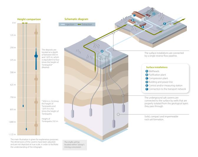
The location of the salt caverns has been selected on the basis of geological studies and corroborated by two independent geomechanical studies, ensuring their suitability and stability during construction and in the operation phase of the underground storage.
